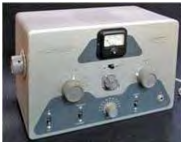
Heathkit DX-20 transmitter covered 80-10 meters, CW only.
