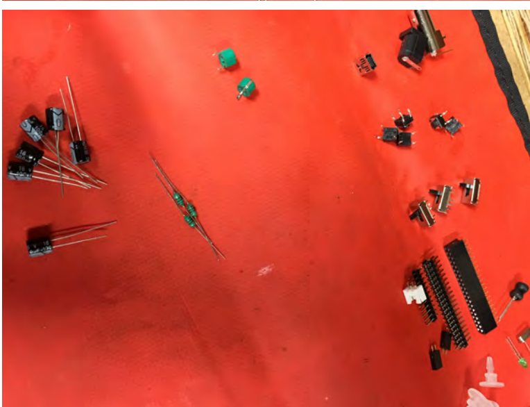
Capacitors are also measured and sorted as well as several inductors and other miscellaneous parts.
