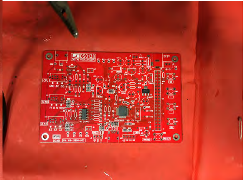
The version of the kit we bought already had the surface mount components on the board.
