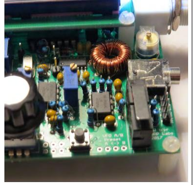
using different types of solder, I ordered a roll of Kester solder core size 66, 63/37 alloy, 0.031 diameter. This works and doesn't leave a lot of rosin residue after you're done soldering. I also used a thinned-out mixture of flux.
